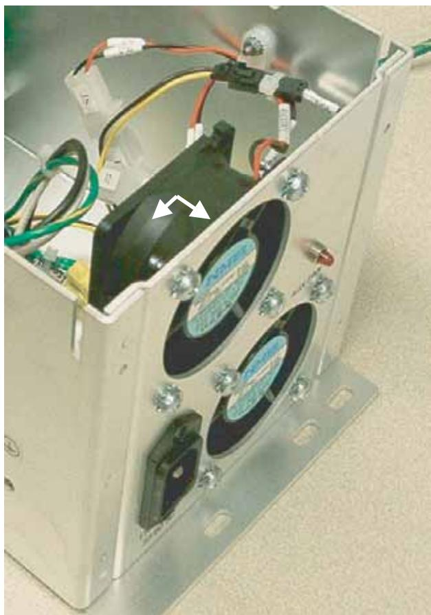
Note the correct orientation for the fan. The fan must be correctly installed to provide the desired airflow.
