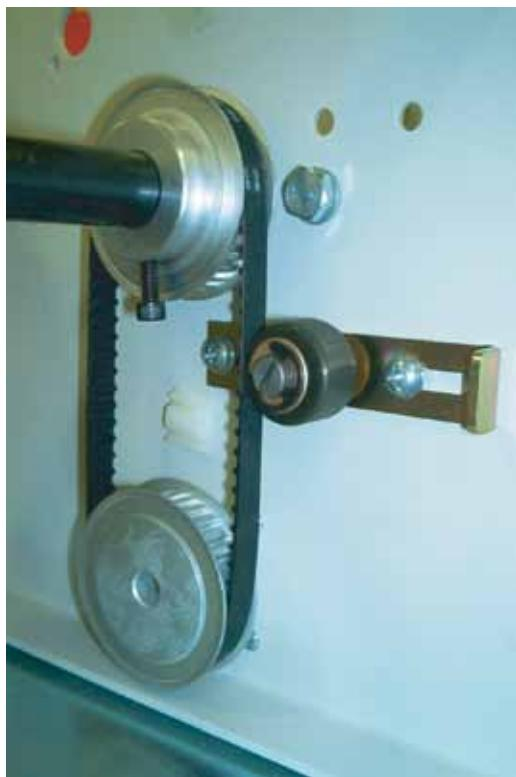
The graphics, (above and left), depict a recently developed encoder tensioner for use on the 10X13 FlowMaster units. The tensioner is similar to the one used on previous Burster units and can be mounted as shown. The unit pictured is not currently released as an assembly, however, all parts can be ordered from Newtown.
