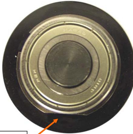
Seat bearing into side plate with the flat spot in the snap ring flush against the deck surface
