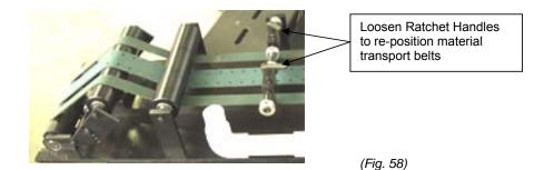
Turn both of the material transport belts guides to the right or left until the guides no longer capture the belts, see figure 59. (Note: It is important to have these guides repositioned to avoid damage to the material transport belts during the re-assembly process)
