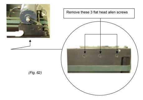
12. Using a 5/32 Allen wrench, loosen (Do not remove at this time) the three (3) flat head Allen screws located at the back motor support, see figure 63. (Note: If these screws are removed, it may not be possible to perform step O.)
