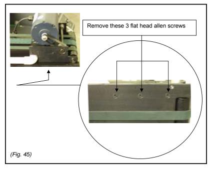
(g) Using a 5/32 Allen wrench, loosen (Do not remove) the three (3) flat head Allen screws located at the back motor support, see figure 46.
