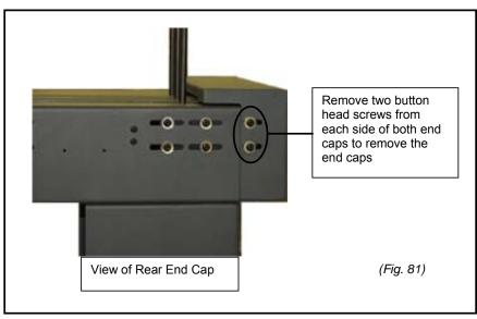
Pull each end cap straight out from the conveyor. (b)
