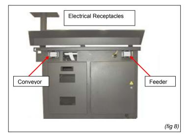
14. Plug the conveyor cable into the receptacle located on the back upper left corner of the ink jet / dryer base, flip up the retaining clips to secure the plug in the receptacle, see figure 8.
