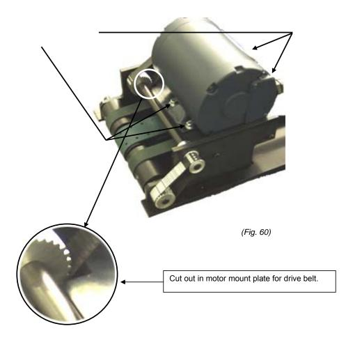
8. Slid the motor towards the drive shaft and remove the drive belt from the drive motor pulley, then lift the motor off of the mounting plate and set it aside, see figure 61.
