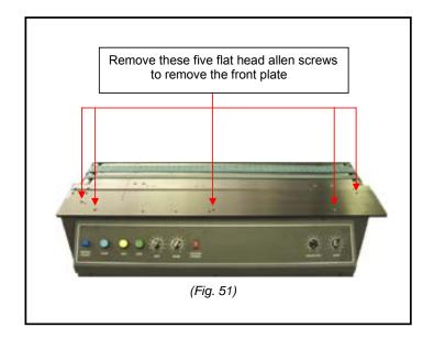
(c) Lift the front plate off of the ink jet base and set it aside.
