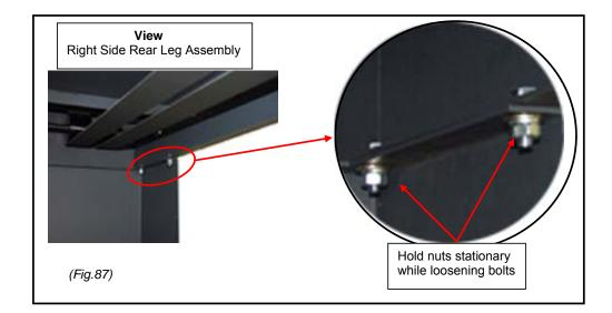
14. Using a 7/16" open end wrench, **remove** the two (2) hex head bolts located under the conveyor bed, found on the left side of the rear leg section, see figure 88. (Note: There is a 7/16" retaining nut under each hex head bolt that will need to be held in place in order the loosen the bolts.)
