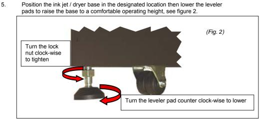
6. Place a level in the center of the ink jet / dryer base and adjust the leveler pads as needed to level the machine at the desired height. Once the machine has been leveled, tighten the leveler pad lock nuts, see figure 3.
