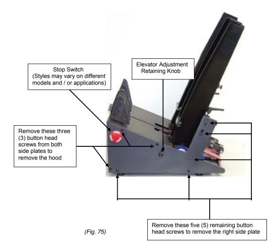
3. Disconnect the wires from the stop switch, located on the right side plate of the feeder, see figure 76.
