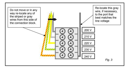
b. Insert the "Dark Gray Voltage Select Wire" in the connection port that is labeled for the best match for the line voltage discovered in step 3, see figure 4. Secure by tightening the retaining screw using a medium tip Philips head screwdriver.
